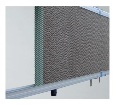
The WDP100-AL water distribution system from Munters provides highly durable means of mounting 100 mm thick CELdek® evaporative cooling pads and supplying water to the pads. Together these form an ideal complete system for incorporating evaporative cooling into the ventilation system of a structure.
